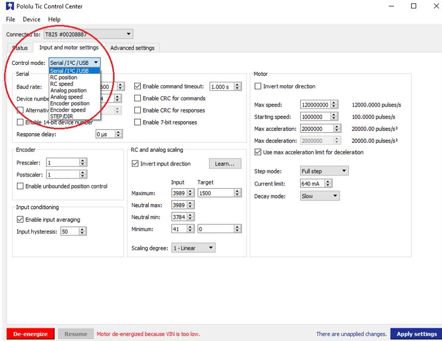
Included in the Quick Start Configuration files are four RC position configuration files (S20-15mm-RC, S20-30mm-RC, S20-50mm-RC, and S20-100mm-RC). The files use the control mode “RC position” to drive the stepper actuator with radio control. The scaling has been predetermined through use of the “RC and analog scaling” block and the “Learn” wizard built into the Tic Control Center software. For explanation on how to use the wizard visit Pololu’s website at <https://www.pololu.com/docs/0J71/4.7>.
