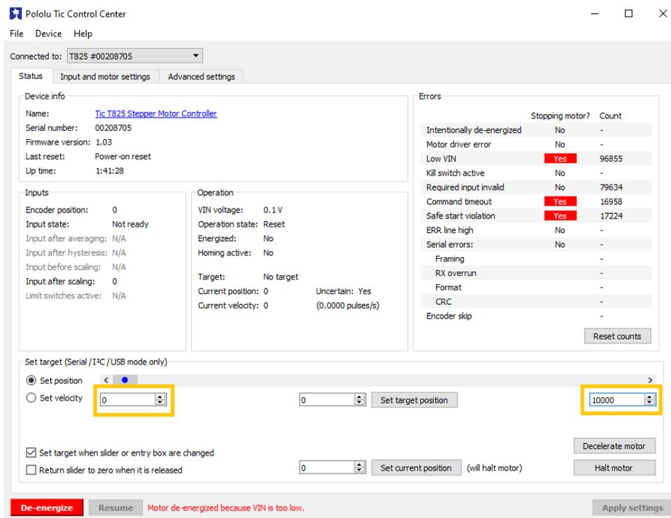
With the correct number of steps inputted you can now move the slide block, however, before it will move the actuator you must first press “Resume” to energize (power) the motor. Actuonix’s linear stepper actuator models do not contain position feedback; this is why it is required to **home** the actuator before use. To **home** the actuator it must be overstepped into either the fully extended or fully retracted position.
