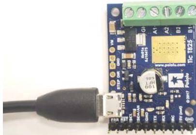
With the Tic Control Center software open and the USB connected, the Tic should automatically connect. If it does not automatically connect then use the drop down menu labelled "Connected to:" and select the Tic. The Tic should now be connected to the Tic Control Center.
