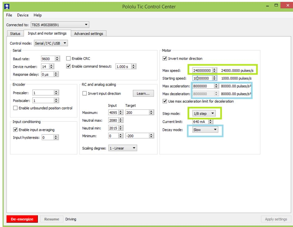
Once the parameters are set it is best to test the travel of the unit using the SLIDE BAR. Only once it is determined to be a successful set of parameters for your application should the control mode be modified.
