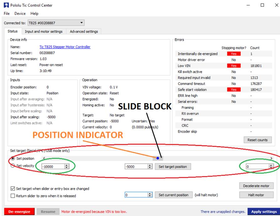
The slide bar represents the actuators stroke, where the slide block is the target position and the position indicator marks the current position. However, as there is no feedback on the stepper actuator if steps are missed the Tic Control Center software does not recognize this and the position indicator will show it has successfully hit the target position.
