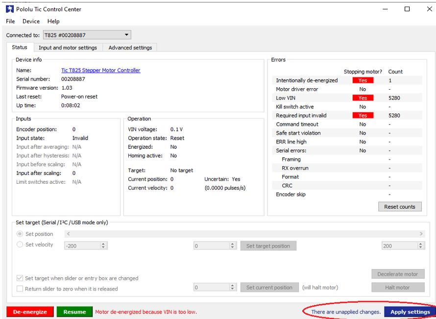
Next is to set the correct number of steps for the actuator to complete a full stroke. Each stroke length has a different number of steps required to travel its entire stroke. The slide on “Status” tab defaults from -200 steps to 200 steps. These values must be changed for the step size and given stroke length of actuator being used.
