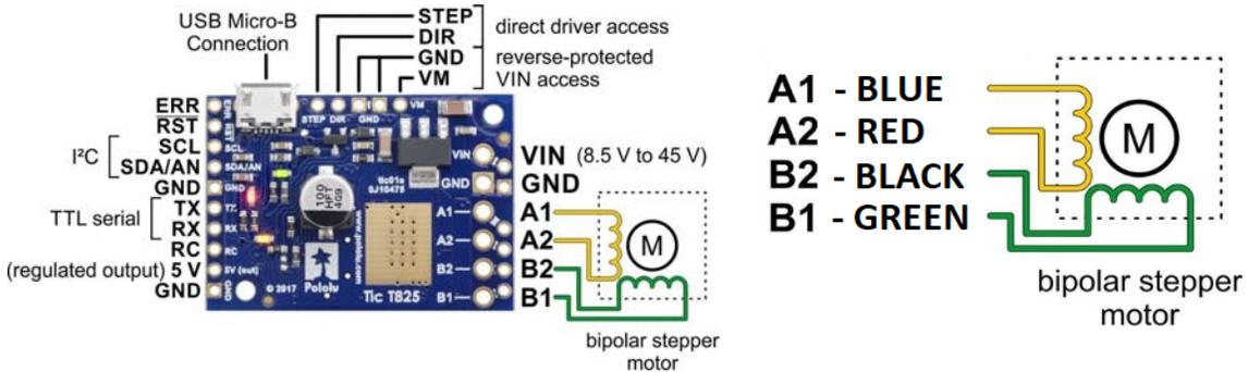
Make sure the stepper motor is connected and the wires are in the correct PIN location.
